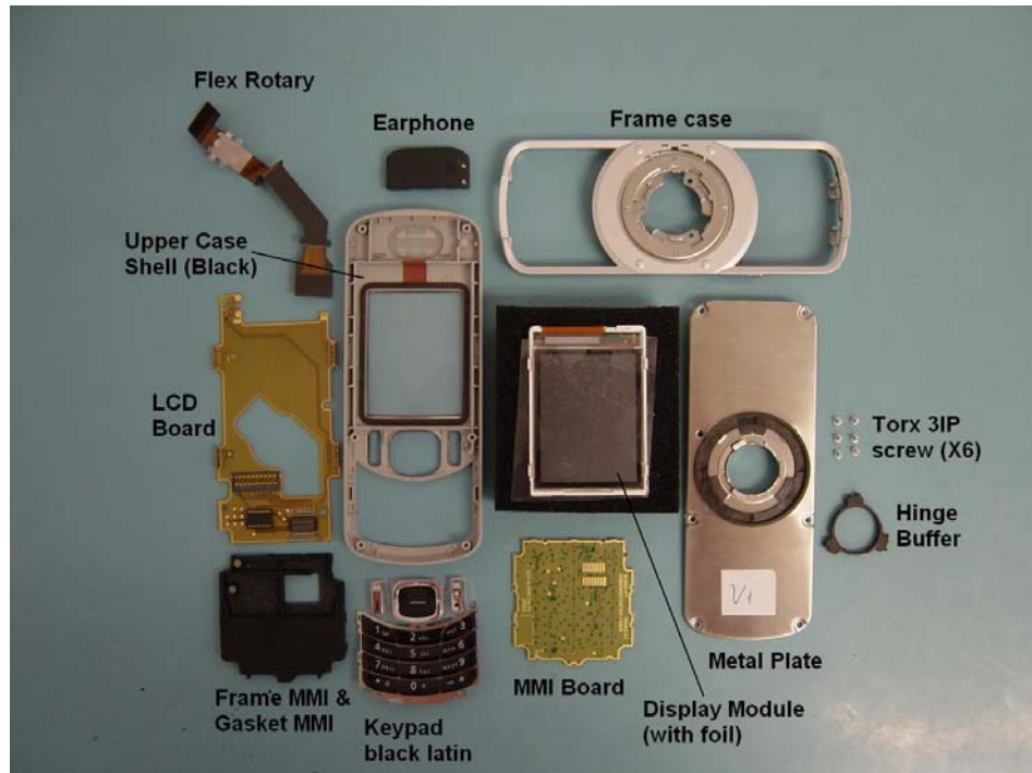
Fully disassembled SK65 (Upper parts)
