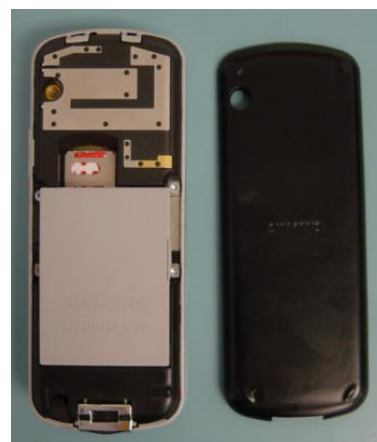
Remove Battery cover.
