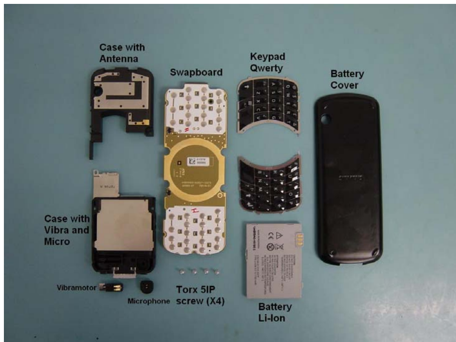
Fully disassembled SK65 (Lower parts)
